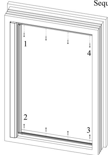
Transfer hole locations for handle and magnet, and use 7/64" drill through first wall of handle bar only.
